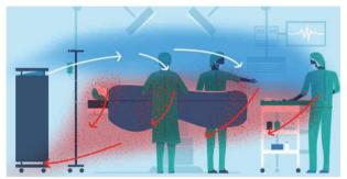
The image above shows a Viruskiller unit controlling the airflow and creating an ideal scenario. The contaminants are constantly being pulled towards the unit by the fan and also pushed down by the clean air above, keeping the breathing zone safe.
